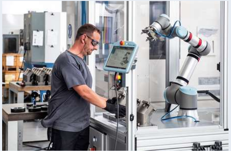
Image 2: Cobots complement human abilities in tasks requiring precision, such as delicate assembly and quality control.
