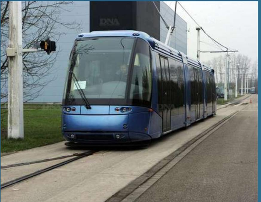
The biggest factors in the emergence of this alternative light rail system are of course the advantages of the rubber wheel. These include being able to climb steeper slopes, lower turning radius, reduced infrastructure and maintenance costs, and braking distance.
