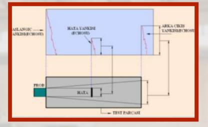
in non-destructive testing applications is extremely simple. As a result of sending ultrasonic sound waves into the material, information about material properties, thickness and discontinuities is obtained. Ultrasonic control has a wide range of applications, from aviation to pipelines, from railways to the manufacturing sector.
