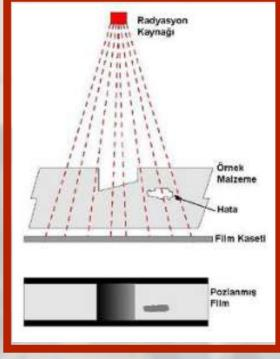
called radiography. This method is applied to ferromagnetic and non-ferromagnetic metals and other materials. X-rays are widely used in non-destructive testing, as they provide the opportunity to examine the internal structures without damaging the materials. Thickness changes, structural changes, errors, assembly details can be detected in materials with X-ray or gamma rays.
