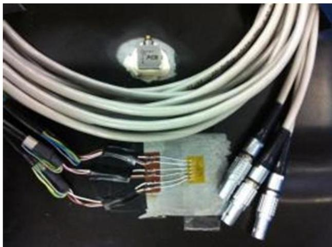
**Fig. 3.** Accelerometer & Strain-gage Instrumentation on the Oil Pan
